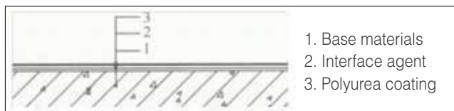
Basic structure of SK one-component polyurea coating
