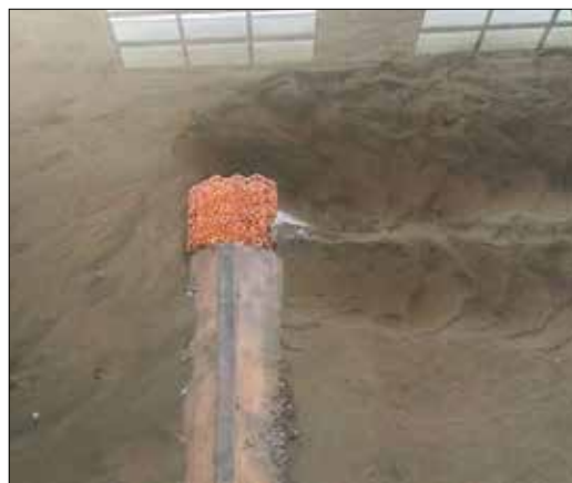
Scouring and silting effect test of permeable dam head, one of the new structures for waterway regulation
